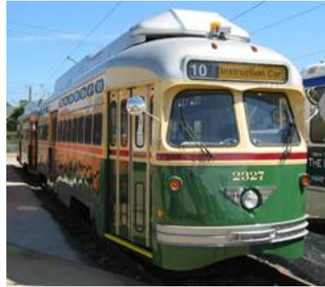
Front of 2327 showing new turn signals.
