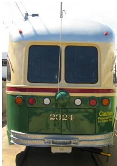
Rear of 2324 showing turn signals, stoplights and back-up lights.
